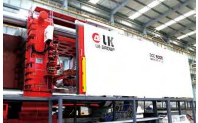
力勁最新研發的6,000噸大型智能壓鑄機可應用至電動車、無人機及航空等層面，配合近年全球工業的趨勢 LK's newly developed 6,000 ton intelligent die-casting machine can be utilised for electric vehicles, drones and aviation, which is in line with recent global industrial trends
