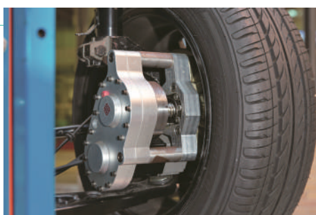
智能純電動防鎖死煞車系統的機電制動器 The electromechanical brake (EMB) of the Smart All-electric ABS
