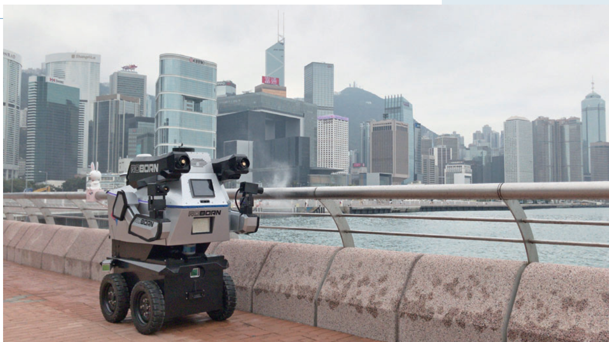
路邦推出5G室外消毒機械人「守護」，可以大範圍、穩定地進行噴灑消毒，現時已應用於本港多個海濱長廊。（受訪者提供圖片） Roborn has launched a 5G outdoor disinfection robots named “Sau Wu”. The robots can spray and disinfect large areas and have already been applied to many Waterfront Promenades in Hong Kong. (Photo provided by Interviewee)
