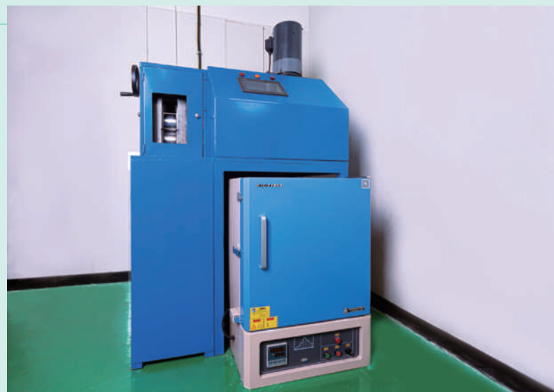
生產力局研究團隊設計出長、闊及高度均少於兩米的軋機，適合寸金尺土的香港使用。 HKPC has developed a new machine, with length, width and height being less than two metres, which is suitable for the manufacturers in Hong Kong with limited factory space.
