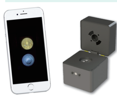
無線珠寶螢光分析儀能將肉眼無法分辨的珠寶及其 贗品區分。 The Wireless Jewellery Fluorescence Analyser can distinguish authentic from fake ones.
