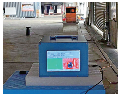
應用於消防的遠程氣體檢測儀（前方）可於安全距離 檢測毒氣和爆炸性氣體。 The Remote Detector for Fire Service can detect toxic and explosive gases from a safe distance.
