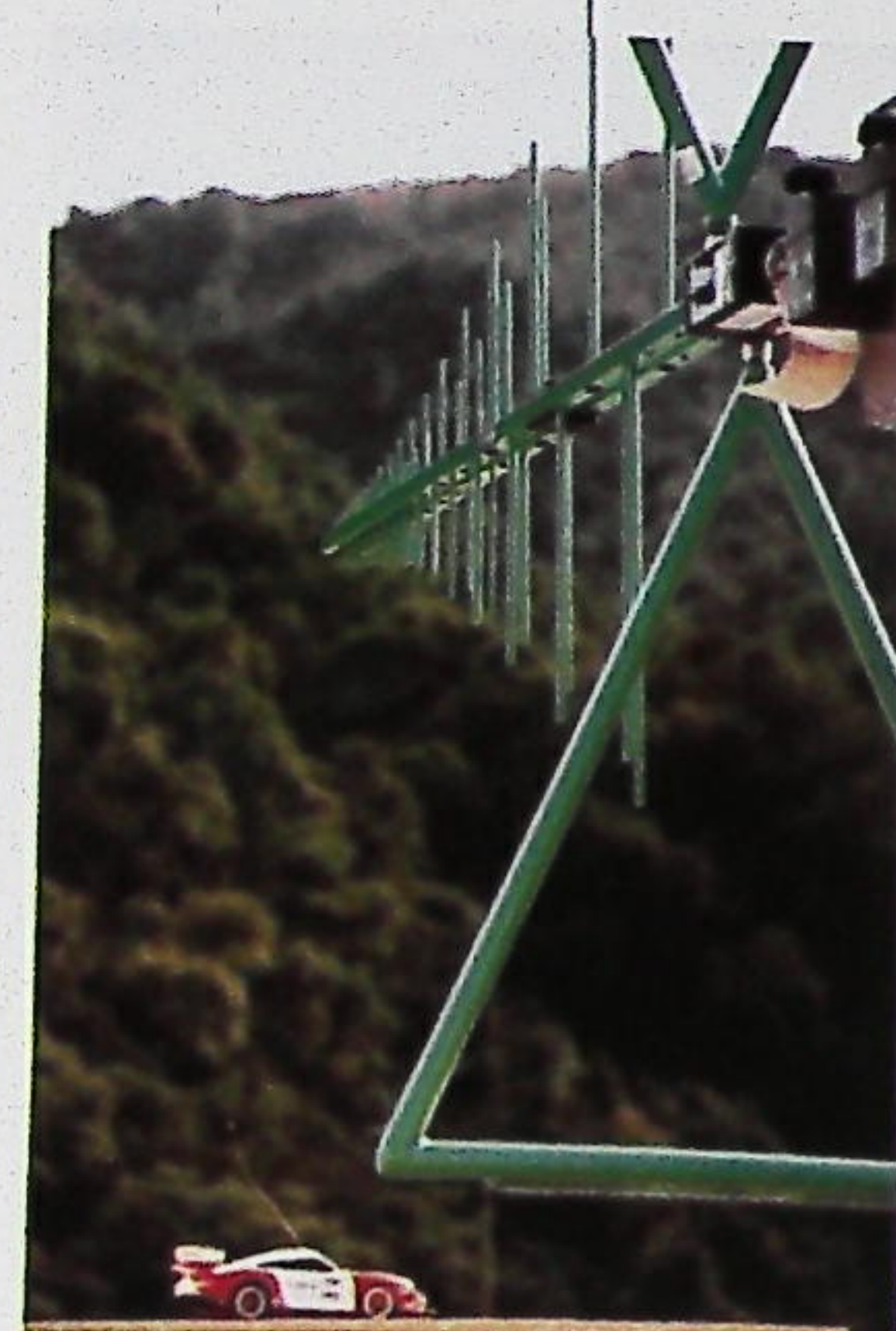
The diagram shows how to measure the radiated emission from the receiver of the electrical toy.
