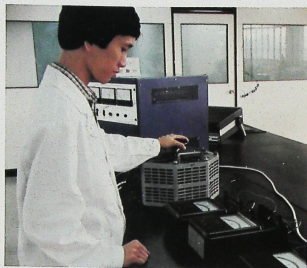
電器之溫升檢定 Heating test and temperature evaluation on electric products.
