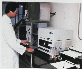
以原子光譜分析儀檢查重金屬含量 Detection of heavy metals by atomic absorption spectroscopy.
