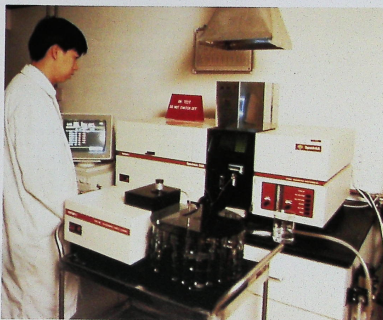
原子吸收光谱分析是本會檢定中心所提供的服務之一。 Atomic absorption spectrophotometric analysis is one of the numerous services provided by CMAA Testing & Certification Laboratories.
