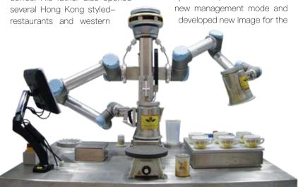
集團與生產力促進局共同研發了一個可自動沖泡奶茶的機器人,預計於今年8月正式面世The group and the HKPC have jointly invented a tea-brewing robot, which is expected to be officially launched in August this year
