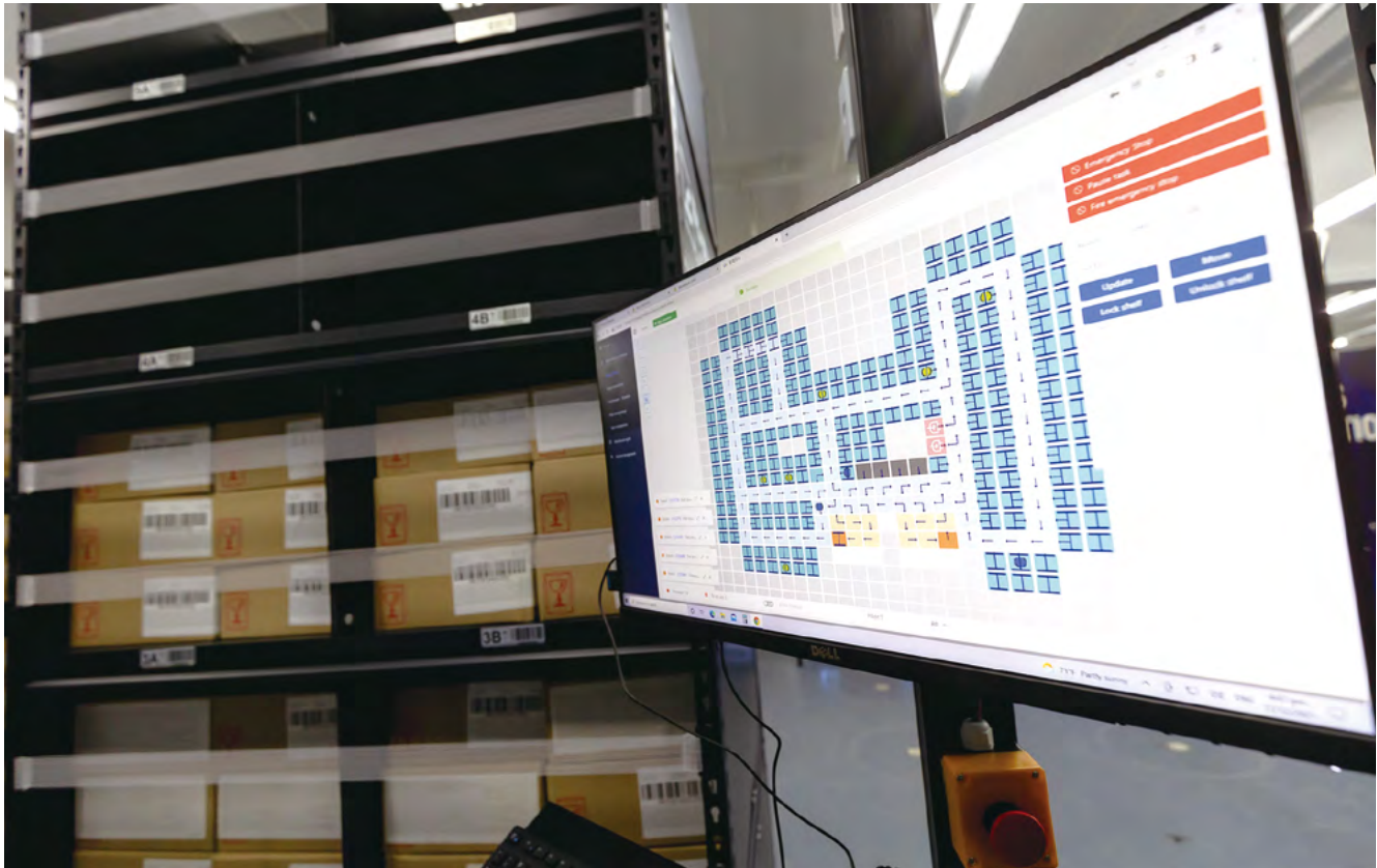
利用人工智能技術，系統會按貨品的熱門程度編排貨架位置，提升揀貨效率 By leveraging AI technologies, goods on shelves are positioned based on popularity
