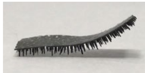
這個極靈敏及多足的軟體機械人，能夠在惡劣的環境下載運重物。 The highly agile, multi-legged soft robot is adaptable to adverse environment and can carry heavy load.
