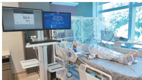
通風系統正在港怡醫院病房進行測試，同時可以量度氣壓、濕度、氧氣量、二氧化碳量等指標。 The fast-track ventilation system is being tested in Gleneagles. Pressure, flowrate, humidity, oxygen and carbon dioxide levels are automatically monitored.
