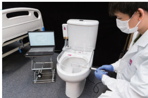
通風系統亦能應用在廁所，可於5秒內把在沖廁過程產生的氣溶膠迅速抽走。 The system can also be used in toilet bowls to extract aerosols generated from a toilet flush in just five seconds.
