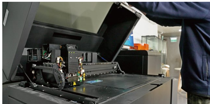
「全彩光敏聚合物噴射技術」3D打印設備可製作精美3D模型。 Exquisite 3D models are made possible with the "Full-Colour Photosensitive Polymer Jetting" 3D printing equipment.
