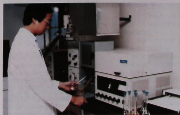
Determination of heavy metals content in paint by atomic absorption spectroscopy 以原子吸收光譜儀分析油漆內重金屬元素含量。
